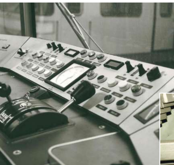
< Drive/brake lever controls v Sanding system from Mödling
